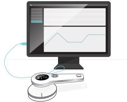
Figure 10. Connect instrument to RaySafe View.
