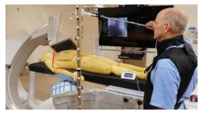
As a basis for product development, the Egg Medical team wanted to understand scatter radiation distribution in the cath lab, so they performed measurements using the RaySafe X2 with a survey sensor. Before the dose exposure study, they validated the RaySafe X2 by comparing ion chamber and solid-state technologies, which showed highly correlated values. They concluded: "RaySafe X2 offers highly accurate dose readings with excellent repeatability."
