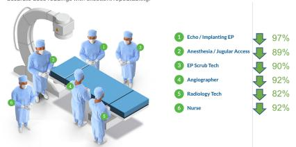
This image shows typical radiation reduction values comparing EggMedical shielding to standard shielding <sup>6</sup>. During test installations in hospitals, each staff member is equipped with a RaySafe i3 dosimeter to monitor their dose in real time. These measurements can be compared with previous values for similar procedures.
