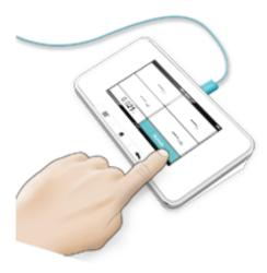
Press Activate to make the instrument ready for measurements.
