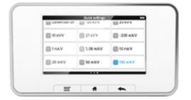
To get other measurement parameters, in addition to voltage (V) and time (s), select an applicable conversion factor. Swipe right from the home screen to access the quick settings with the conversion factors.
