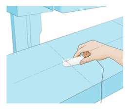
Place the connected sensor centered in the field with the crosshair towards the X-ray source. The angle of the sensor in the horizontal plane has no impact on the measurement result.
