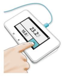
The sensor is constantly measuring. If you want to store a value, press the button once the reading is stable. The measurement will continue below the stored value. **Tip!** Tap a parameter to get large digits and parameter information. Switch between these by swiping sideways.
