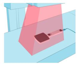
You can also use the sensor for low dose rate measurements, positioned centered in the X-ray field, with the dark side towards the radiation source.
