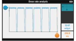
Slide the handles to view, for example, the peak dose rate of a pulse. Pinch with two fingers to zoom in the waveform area.
