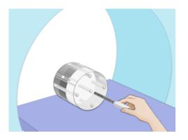
Push the connected sensor tight into the phantom  $\ldots$
