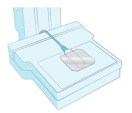
Place the sensor centered and 6 cm from the chest wall. Place the 2 mm Al filter on the sensor. Be sure to cover the active sensor area.
