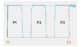
T: Time P1, P2, P3: Pulses kVp: Peak tube voltage
