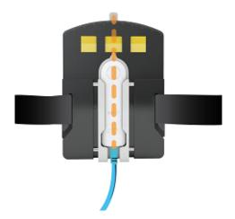
Position the panoramic holder with the X2 sensor centered, with the whole sensor rectangle inside the direct beam.
