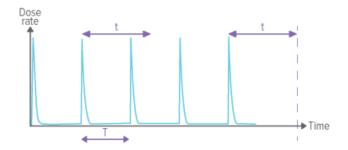
Stop delay setting longer than the time between pulses (t>T), will result in one long measurement. Note that you have to wait as long as the stop delay setting (t) after the last exposure before the measurement ends and values will be displayed.
