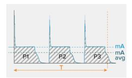
T: Time P1, P2, P3: Pulses mA: mA mA avg: mA value if the setting mA mode is mA avg : Displayed mAs value.
