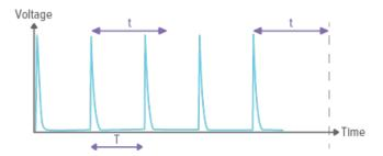
Stop delay setting longer than the time between pulses (t>T), will result in one long measurement. Note that you have to wait as long as the stop delay setting (t) after the last exposure before the measurement ends and values will be displayed.
