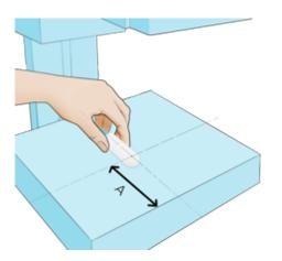
The MAM sensor is ready to measure dose and HVL for all anode/filter combinations without changing any settings. Place the connected sensor centered in the field, with the crosshair 6 cm (4 cm in the US) from the examination table front edge (A). The angle in the horizontal plane has neglectable impact on the measurement result.
