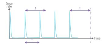
Stop delay (t) setting longer than the time between pulses (t>T), will result in one long measurement. Note that you have to wait as long as the stop delay setting (t) after the last exposure before the measurement ends and values will be displayed.
