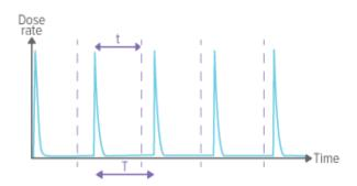
Stop delay setting (t) shorter than the time between pulses (t<T), will result in many short measurements (one for each pulse).
