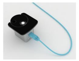
**Illuminance:** Place the connected sensor with the diffuser in the direction you want to measure, and with illuminance selected on the sensor wheel.
