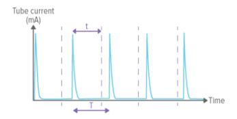
Stop delay setting shorter than the time between pulses (t<T), will result in many short measurements (one for each pulse).
